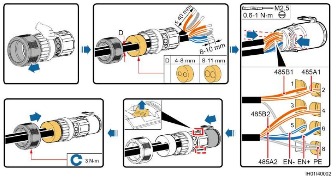
**Figure 5-20** Assembling a signal connector (ALARM port)
