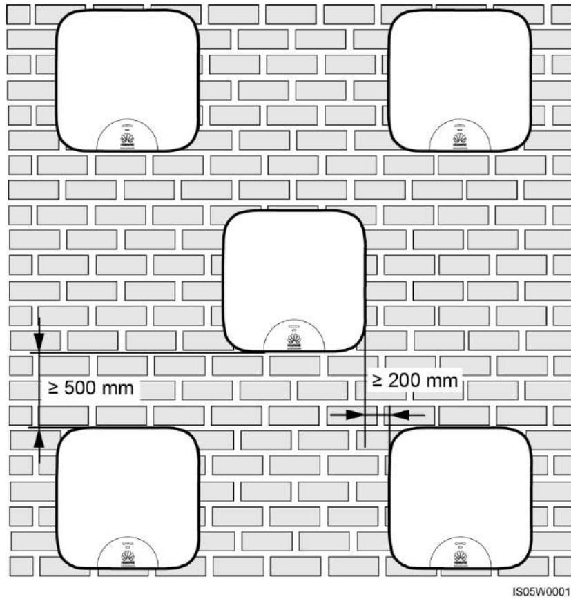
**Figure 4-5** Stacked installation mode (not recommended)
