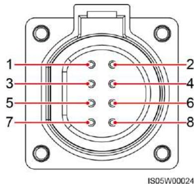
The COM port provides two RS485 communications ports and one enable signal port to connect to power collectors, batteries, and so on.
