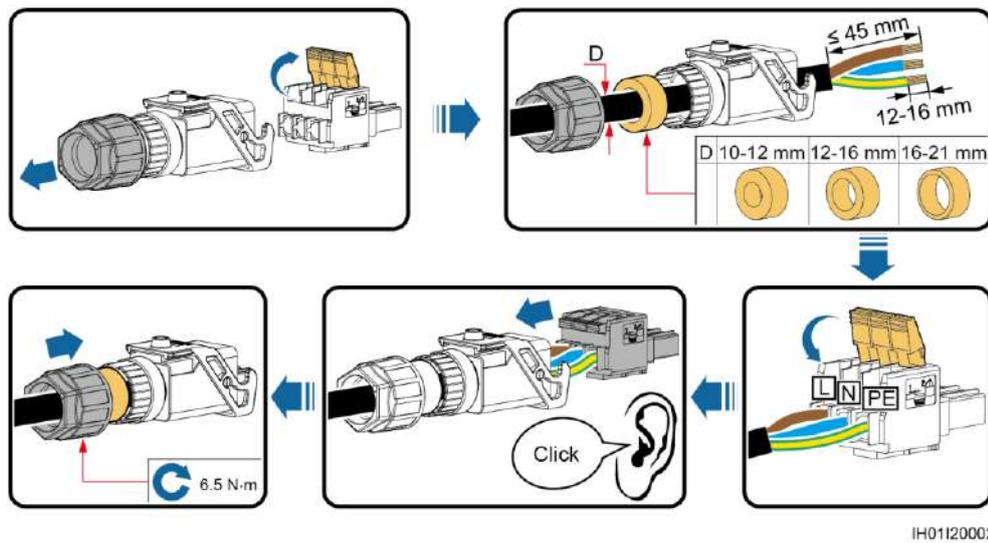
**Figure 5-6** Assembling an AC connector (two-core wire)
