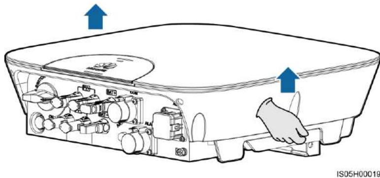
**Step 2** Install the SUN2000L on the mounting bracket and align the SUN2000L enclosure with the mounting bracket.
