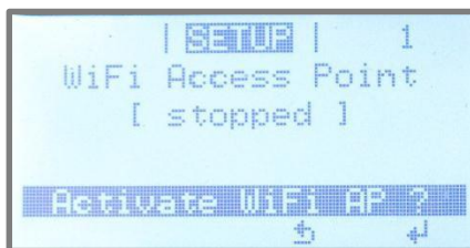
Fig.1: Activating the WiFi access point on the Inverter's display - Setup menu
