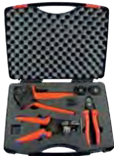
Assembly case I » Four-mandrel crimping pliers PEW 8.76 with locator » Cable shears to 50.0 mm² » Stripping pliers 2.5 to 10.0 mm² (72 01 67)
