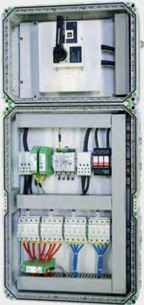
HISbox® Monitoring 8 generator connection box +/- fuse / surge protection 2 / DC-DC power / LWL repeater / 160 A
